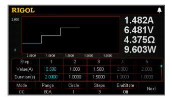
You can generate complex sequences by editing the setting value for each step, the dwell time, and slew rate (the slew rate can only be edited in CC mode) to meet the complex test demands.
